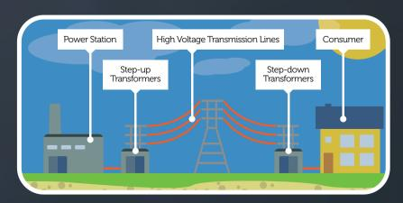
The transfer of electrical energy via the grid is very efficient. When currents in a cable are higher, more energy is dissipated to the surroundings through heating. As high currents waste more energy than low currents, electrical power is transported around the grid at a high voltage and low current.
